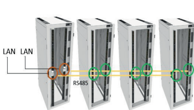
Deployment illustration with one daisy-chain on feed A and one daisy-chain on feed B
